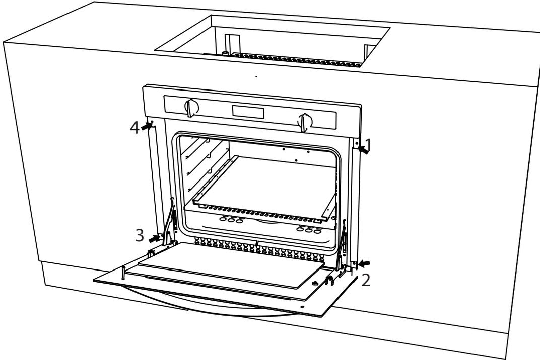
STEP 4 - Slide the vent assembly over the oven outlet flange
