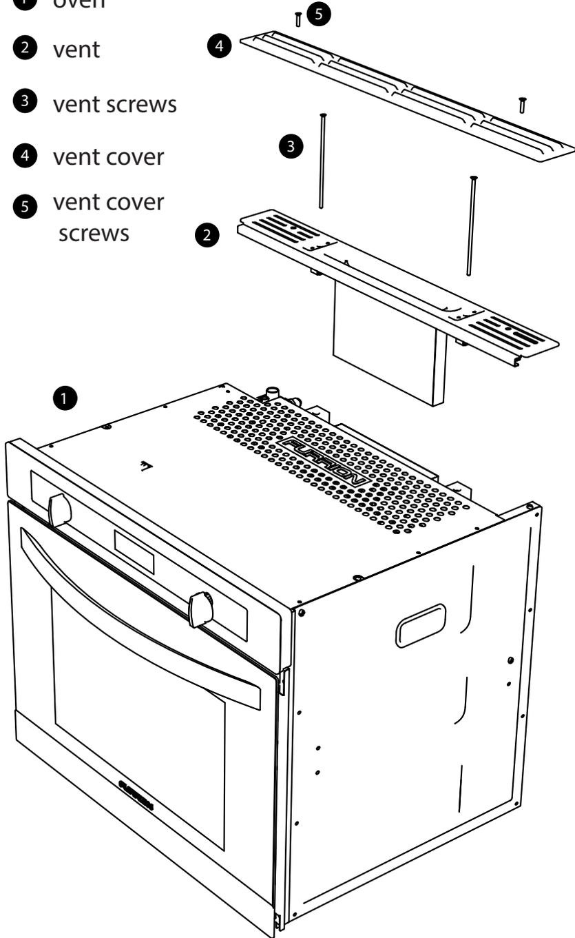
STEP 2 - Push the oven into the cut out perfectly and then connect the gas pipe & 12V power.
