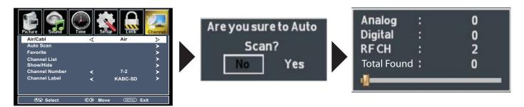
Select Air when TV is connected to an indoor / outdoor antenna.
