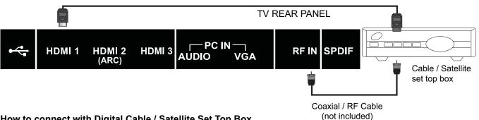
How to connect with Digital Cable / Satellite Set Top Box
