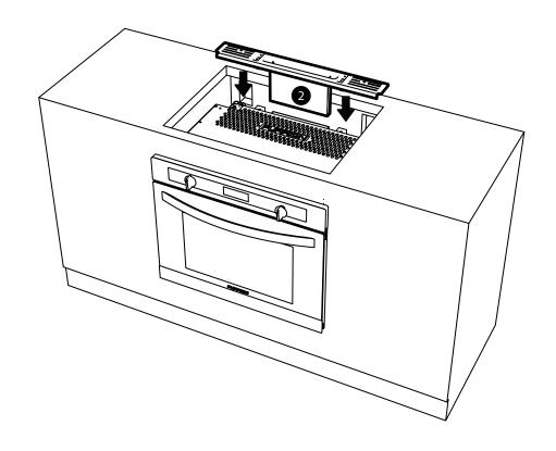
STEP 5 - Install 2 vent screws to secure the vent
