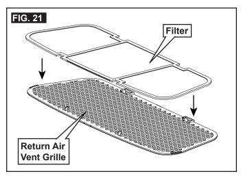
6. Install return air vent grille into the air distribution box. Slide return air grille tab into slot in ADB and rotate up and snap in place. See (FIG. 22). Installation
