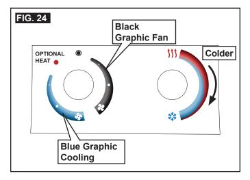
2. The Thermostat controls the temperature range at the filter between approximately 65° F and 90° F.
