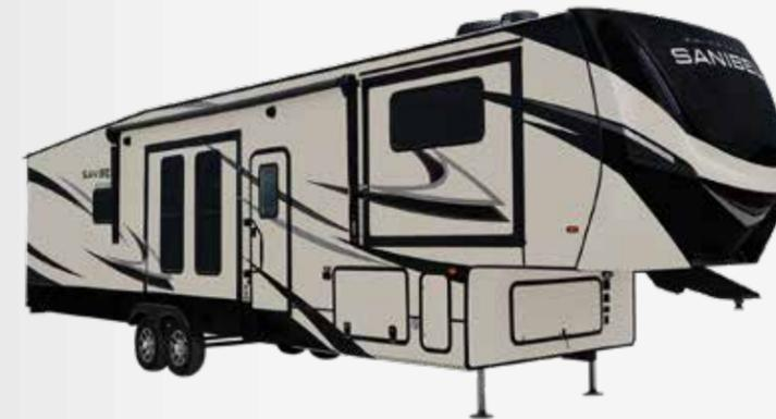
**UVW (Unloaded Vehicle Weight)\*** is the typical weight of the unit as manufactured at the factory. It includes all weight at the unit's axle(s) and tongue or pin and LP Gas. The UVW does not include cargo, fresh potable water, additional optional equipment or dealer installed accessories. \*Estimated Average based on standard build optional equipment.
