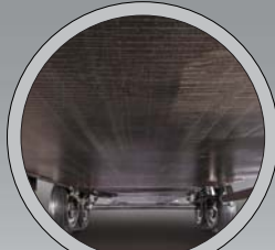
FULLY ENCLOSED UNDERBELLY AND GATE VALVES
