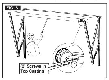
4. AWARNING IMPACT OR PINCH HAZARD. Hold pull strap firmly before removing screw(s) at top casting. The fabric roller tube is under spring tension, which will attempt to close the awning quickly and unexpectedly. Failure to obey this warning could result in death or serious injury.
